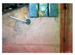
5. From inside the engine compartment, insert the release rod through the rubber grommet (the rod end with the 90° bend). Lift the release rod, twist 90° anti clockwise and hook the release rod through the small hole in the release
