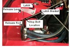
For TR6 applications, the release hook will fit between the main latch and the safety catch loop.
